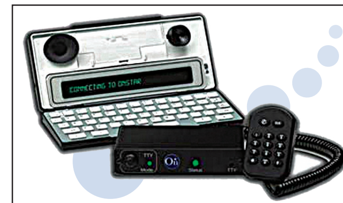
Portable automotive TTY equipment, like this system from Onstar, allows deaf, hard of hearing and speech disabled auto owners to access their car's built-in communications system.
